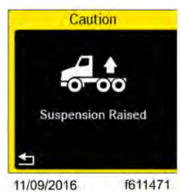
Fig 64, Suspension Raised Alert - ICUC
