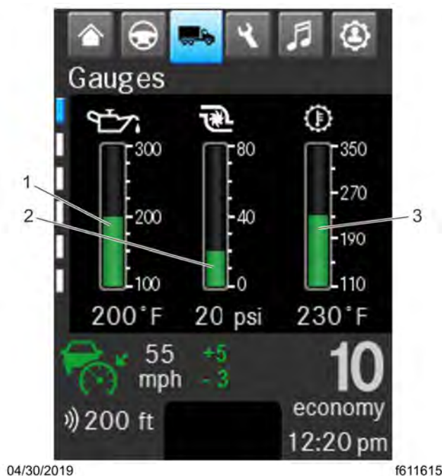
Fig 59, Digital Engine Oil, Turbo Boost Pressure, and Transmission Oil Temperature Gauges - ICUC
