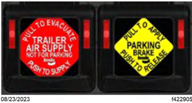
Fig 260, Tractor Parking Brake Set and Trailer Spring Brakes Set
