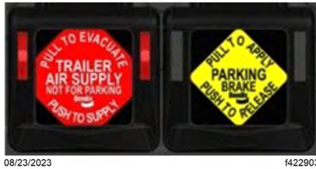
Fig 258, Tractor Parking Brake Released, and Trailer Spring Brakes Set
