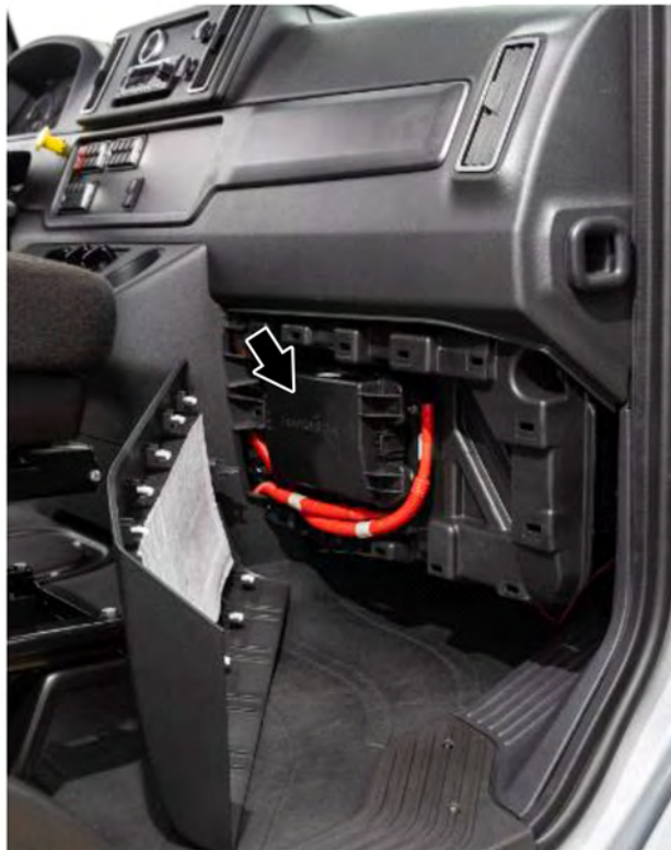
Fig 230, Power Distribution Module (PDMi) Behind Right-Side Dash
