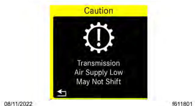
Fig 309, Low Transmission Air Pressure Pop-up
