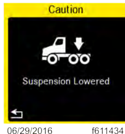
Fig 63, Suspension Lowered Alert - ICUC
