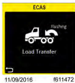
Fig 66, Load Transfer Alert - ICUC
