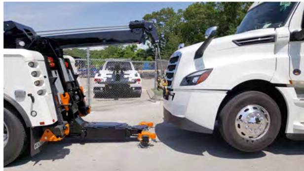
Fig 415, Moving the Stinger and Crossbar Under the Bumper
