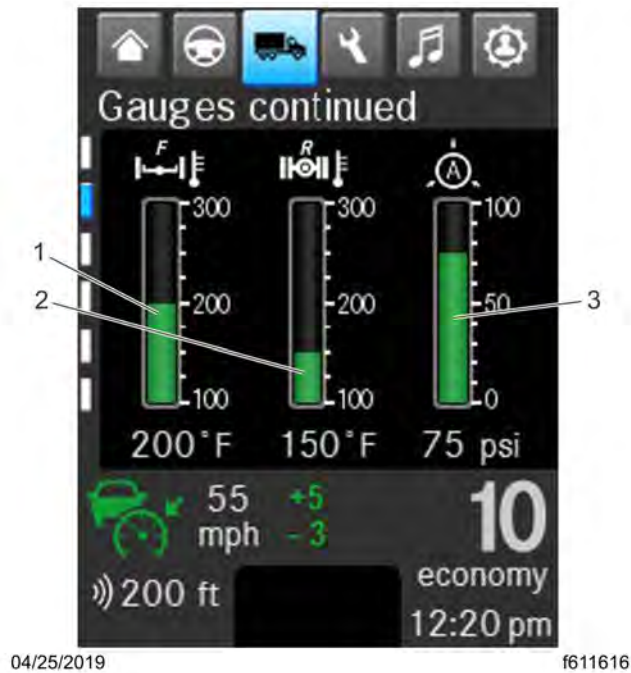
Fig 56, Digital Front and Rear Axle Temperature, and Application Air Pressure Gauges - ICUC
