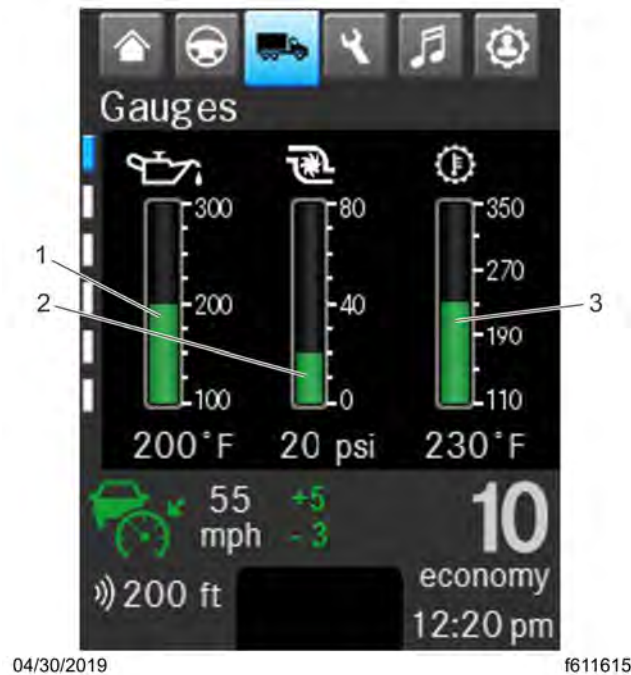
Fig 58, Digital Engine Oil, Turbo Boost Pressure, and Transmission Oil Temperature Gauges - ICUC
