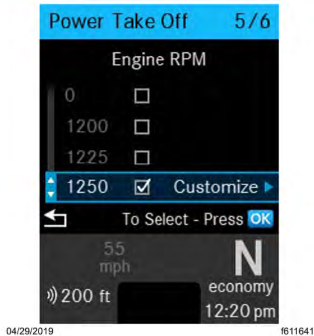
Fig 52, Quick Access Screen: Power Take Off (PTO)
