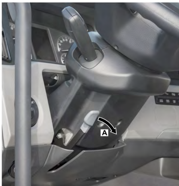
Fig 87, Unlocking the Steering Column
