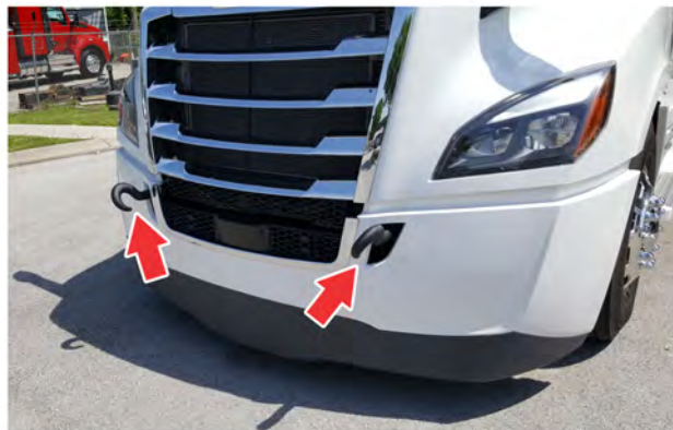
Fig 412, Tow Hooks Installed, Facing Down
