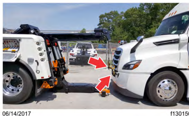
Fig 414, Tow Cables Connected to the Tow Hooks
