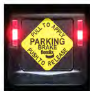
Fig 254, Parking Brake Set Status After Startup
